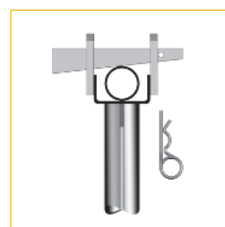
Detail for roof support
