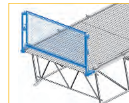
Side protection, eaves
