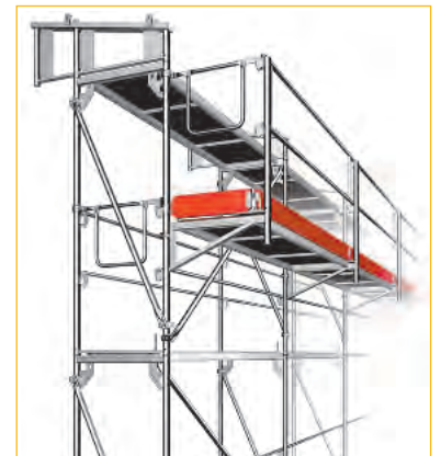
Top scaffolding guardrail, secure assembly thanks to lower bracket levels
