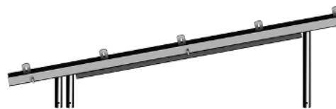
▶ Half coupler for roof support for pedestrian tunnel
